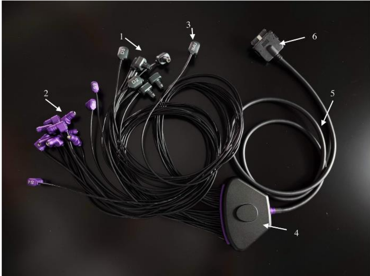
Fig. 2. Optode bundle (PN: SPE-021): 1. Infrared light detectors, 2. Dual-band infrared light emitters (LEDs), 3. IMU module (Accelerometer and gyroscope sensors), 4. Breakout module, 5. Cable, 6. Connector.
