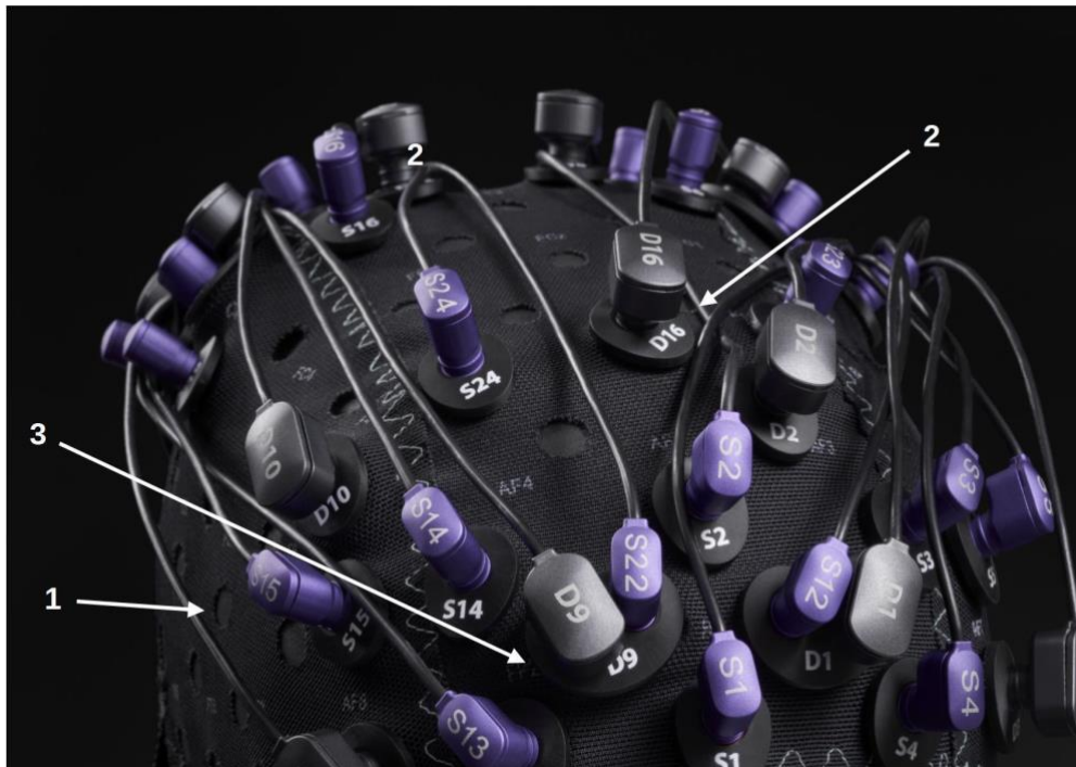
Fig. 3. Textile Cap (PN: SPE-CAP): 1. Holes for mounting optodes, 2. Optode mount for single emitter/detector, 3. Double optode mount detector and short-channel emitter.
