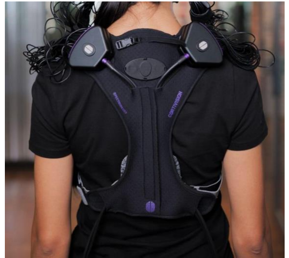
Fig. 9. Harness (PN: SPE-HM1) for attaching the amplifier (1) and cable management (2).
