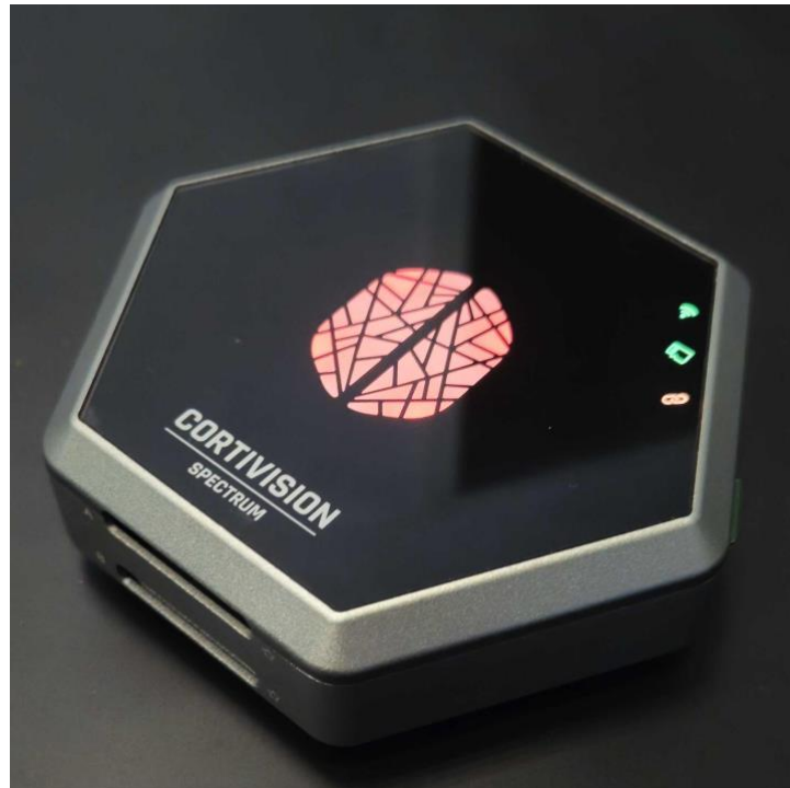
Fig. 16. Marks on the housing and connector (1). The red LED on the housing indicates incorrect connection of optode bundles to the amplifier (2).
